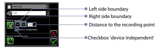
If a device is connected, you can allow recording dependent of the device. In this case the boundary will be recorded while the device is in work.
